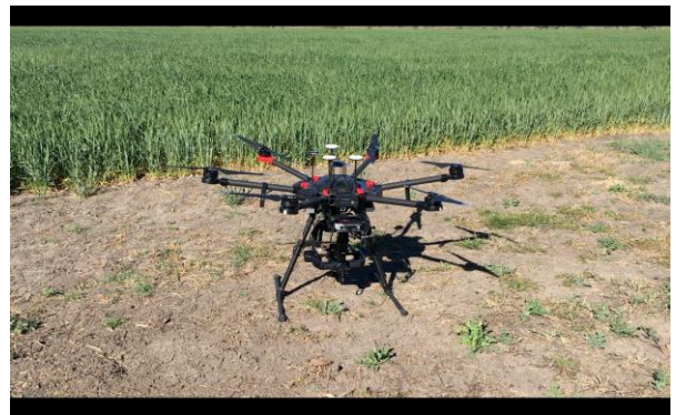
FluroSat uses a drone with a hyperspectral camera to scan crops and collect data.
